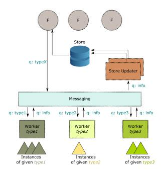
Figure 2. Architecture of the dynamic Software-as-a-Service
